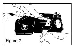
Continue pushing the blade until it reaches the blade holding pin. Lift the blade over the blade holding pin using a finger or a screwdriver for additional leverage (Figure 2).
