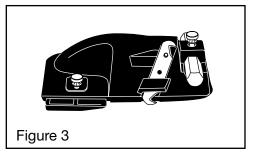
Push the blade over the blade holding pin until the blade holding pin inserts in the top hole of the blade (Figure 3).
