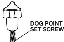
**USE THREE ARM KNOB PROVIDED WITH DUST COVER. DOG POINT SET SCREW IS EASIER TO INSERT.**
