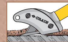
POINT LIFTS CARPET TO THE BLADE
