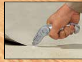
CUT VINYL & LINOLEUM
