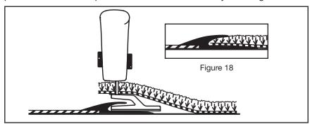
INSTALLATION TIPS: Glue carpet within two feet of the molding.
