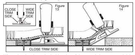
When trimming, keep the inside edge of the cutter's base pressed tight against the Z-bar. This will give you the perfect amount of carpet to fold underneath the Z-bar once the trimming operation is complete.
