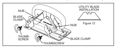
Note that on the base there is a "close trim side" and a "wide trim side" (Figure 13). The close trim side is for trimming Z-bar that is being installed adjacent to a low elevation surface (Figure 13). The wide trim side is used when installing carpet adjacent to an elevated surface, requiring the trimmer to be tilted over (Figure 14).
