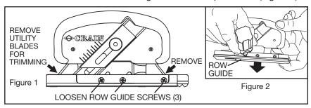
Part the nap of the carpet with a row finder or separator. Set the base of the cutter on the carpet with the extended row guide (Figure 3) inserted into the parted row (Figure 4). With some downward pressure on the handle of the tool, press the row guide down (Figure 3) to the bottom of the row. Once the row guide depth is set, retighten the 3 screws.
