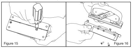
Loosen the two thumbscrews, which loosens the blade clamps. Install two utility blades as shown in Figure 17.
