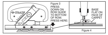
NOTE: The row guide should ride on the bottom of the row when the base is flat on the face of the carpet (Figure 4). The base should not teeter back and forth on the row guide. If it does, shorten the depth of the guide until there is no rocking, yet the guide still contacts the bottom of the row.
