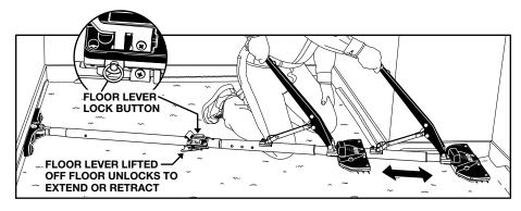
The Lever Extension Tube can be extended or retracted by raising the floor lever off the floor. Note: the floor lever lock button must be pulled to the OUT position.
