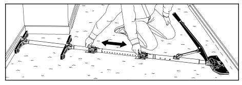
The Lever Extension Tube can be extended or retracted from the tail by raising the hand lever. The tubes will also always extend automatically if they are pushed backward.
