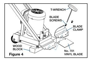
NOTE: Crain blades with slots can be changed by loosening blade screws a few turns, pulling out previous blade, then installing the new blade. The blade screws and blade clamp do not need to be fully removed.
