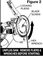
Hold onto the plastic housing, then push hard on the hex wrench counter-clockwise to open. If the blade is very hard to remove, use a pair of locking pliers to hold the blade, and add an extension tube on the hex wrench for extra leverage.
