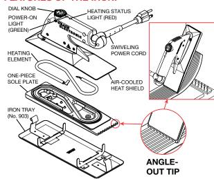
**Electronic Temperature Control:** Set a desired temperature on the dial between 240°F and 420°F and this iron will maintain that temperature continuously +/- 15°F. Initial overshoot and subsequent swings in temperature are reduced by this iron's highly sensitive thermistor and responsive digital control board. For your reference, ten temperature settings are marked on the dial corresponding to temperatures between 240°F and 420°F.
