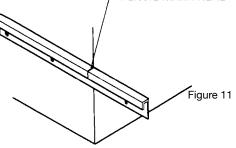
**2.** Place wall leg on flat die shoe, and make a cut at the mark (see figure 12).
