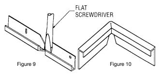
CARPET CAP: Please note that inside corner on carpet cap can be butted, or use a miter box to make 45° corners, as this tool will not do the job adequately.
